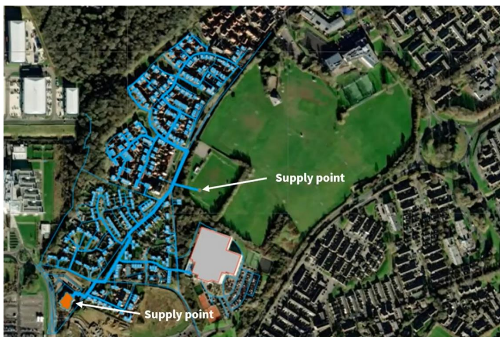
Figure 36. THERMOS, Heating network route optimization.
