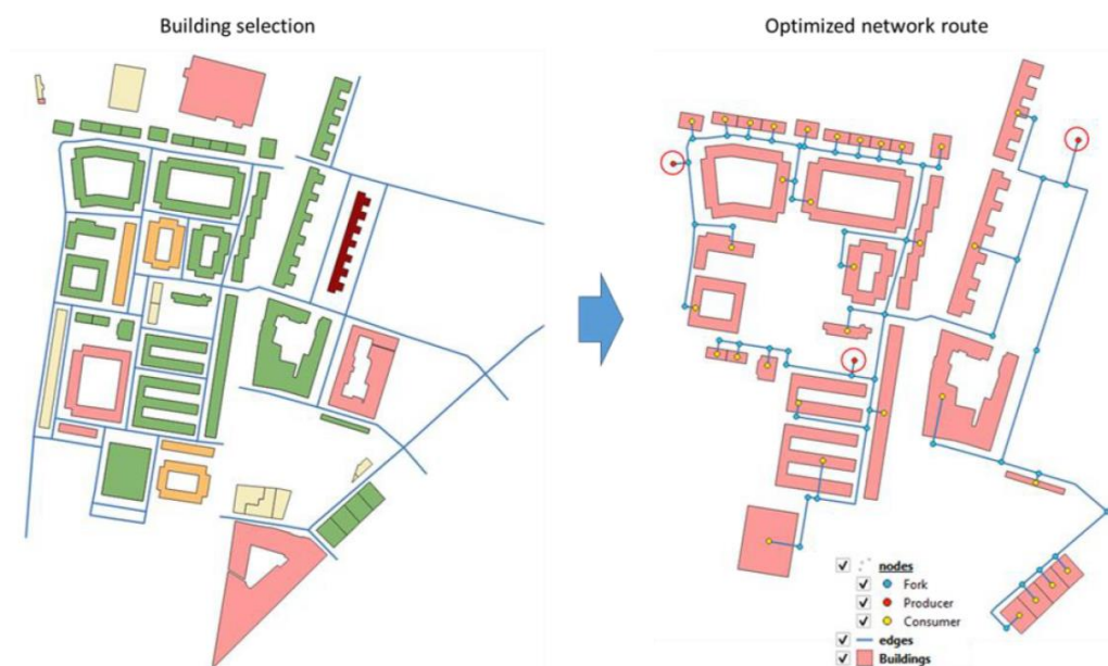
Figure 22. Example of the inputs and route optimizer of Rewardheat [34]
